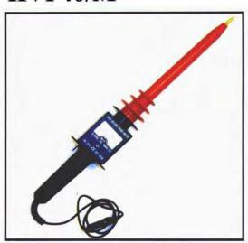
Maximum Input Voltage: 40KVDC Positive or Negative Polarity
